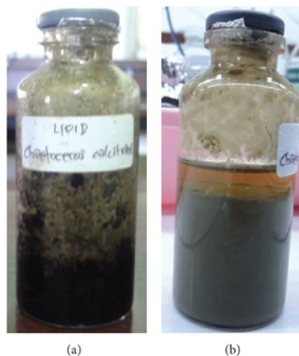
FIGURE 2: (a) Lipid of phytoplankton Chaetoceros calcitrans . (b) Result of transesterification reaction.
